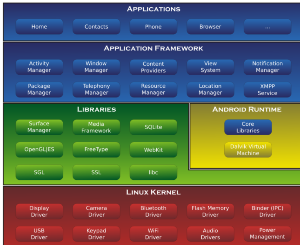
Figure 3.1: The Android Software Stack
